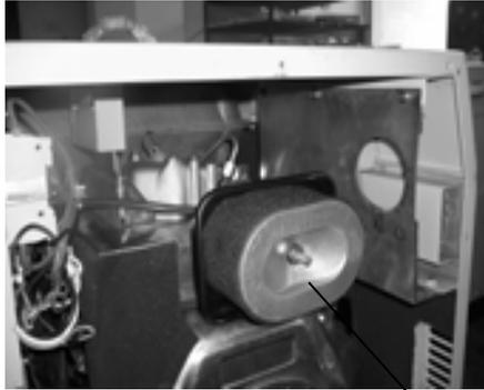
(1) Loosen the butterfly nut, take the cover of the air filter off and take the air filter element out.
